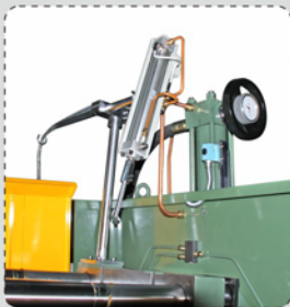
Pneumatic Sweeper for casting removal
